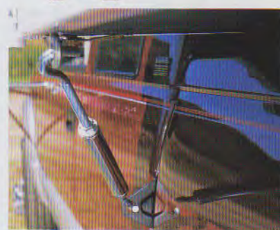
Happijac® chrome-plated anchors are recommended to attach the camper to the truck. The front anchors are spring-loaded to absorb unexpected bounces and are designed to attach to the front of the truck bed with special plates. Rear tie down attaches at bumper. They're proven to be the safest and strongest camper tie downs and turnbuckles on the market.
