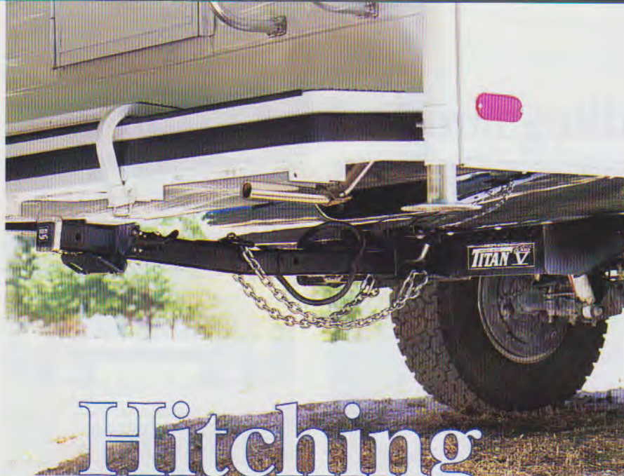
TITAN Class V Receiver with 2-1/2" tube steel extension bar.
